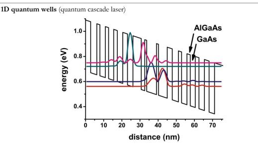
Conduction band structure of a quantum cascade laser including the most important electron wave functions.
