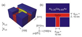
The figure on the left (a) shows schematically the conduction band profile of a T-shaped quantum wire. The schematic on the right (b) shows the relevant dimensions and materials.
